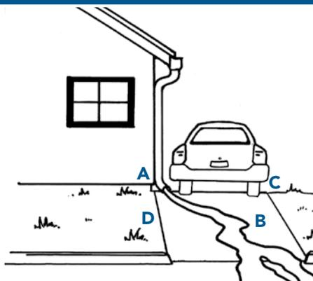
**B** This driveway slopes toward the street and creates runoff potentially contributing to flooding, erosion, and pollutants in nearby storm drains and streams.
