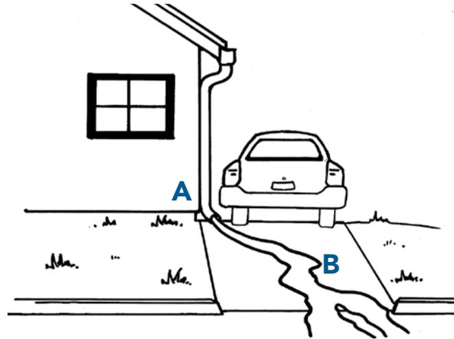
**A** The downspout is directed toward an impervious (concrete) driveway that drains to the street. The resultant runoff may damage roads, exacerbate downstream flooding, or carry pollutants to nearby waterways.
