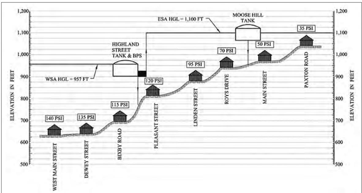
Figure No. 3 – Hydraulic Profile Two Pressure Zones
