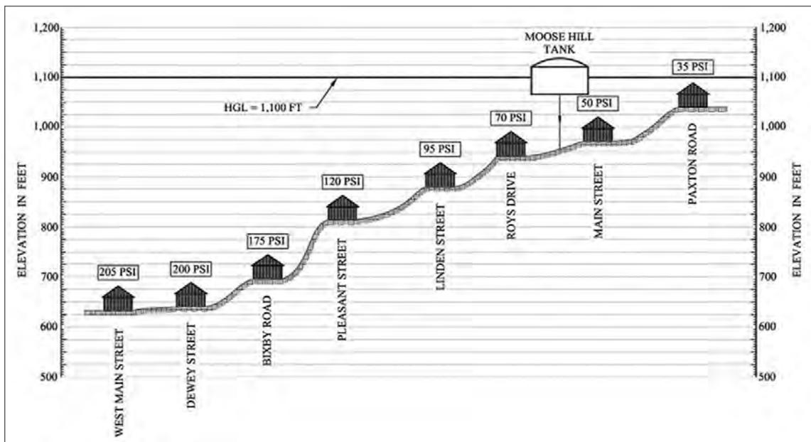
Figure No. 1 – Hydraulic Profile One Pressure Zone
