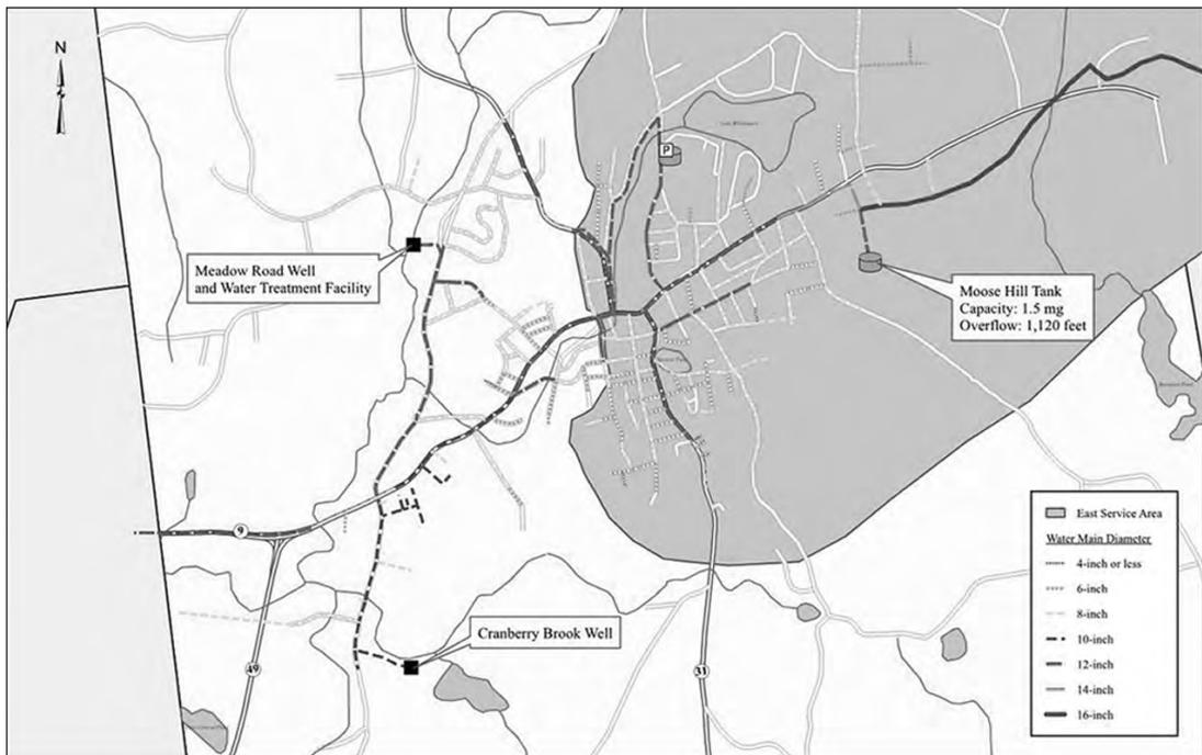
Figure No. 2 – Two Pressure Zone Separation Boundary
